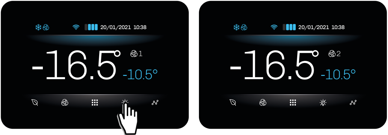
Fig. 32. Switching cold room light on/off
