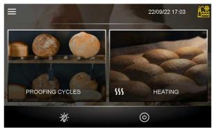
To switch the device on, press the central key on the stand-by screen; to switch the device off, press the key on the lower part of the Home screen.
