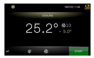
The values of the temperature setpoint and fan speed can be changed before starting up the desired cycle; if a timer is not set to end the cycle after the pre-determined time, the cycle will continue indefinitely.
