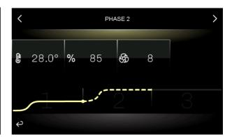
Temperature regulation is active and has a neutral zone adjustment, the working setpoint is set by the end user. Moving from the reawakening setpoint (previous phase) to the proofing setpoint can be gradual, with the incremental percentages set while the parameters are being set (parameters rL0 - rL10).
