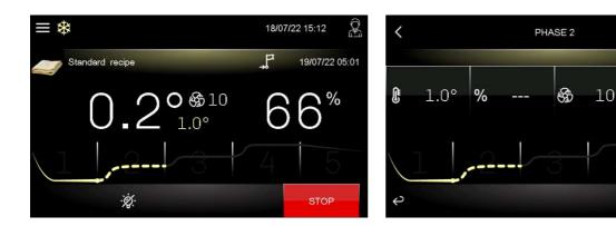
Temperature regulation is active and has a neutral zone adjustment, the temperature setpoint, humidity setpoint (if control of this is required) and fan speed are set by the end user.
