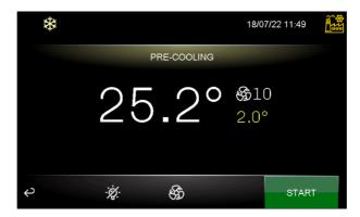
When the cycle has been activated, the controller automatically goes to the main page and displays the cabinet temperature and the setpoint to reach in the place of the pre-cooling key.
