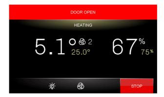
When the alarm bar is pressed, the buzzer will be silenced and the controller will automatically go to the ALARM LIST screen, where only the active alarms will be displayed:
