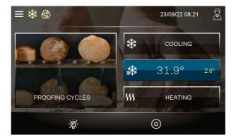
When it reaches the temperature setpoint for the first time, the buzzer will sound. If the temperature in the cabinet is equal to or lower than the setpoint, the pre-cooling function cannot be activated.
