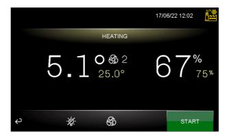
Before starting up the desired cycle, the values of the temperature setpoint, humidity setpoint and fan speed can be changed; if a timer is not set to end the cycle after the pre-determined time, the cycle will continue indefinitely.
