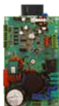
Easy Compact inverters for asynchronous and synchronous motors 1500 W @ 230 VAC Inverter Easy Compact per motori asincrono e sincrone - 1500 W @ 230 VAC
