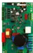
Easy Compact inverters for asynchronous and synchronous motors - 750 W @ 230 VAC Inverter Easy Compact per motori asincrono e sincrone - 750 W @ 230 VAC
