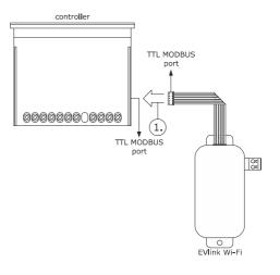
Connect the TTL MODBUS port on the EVlink Wi-Fi to the TTL MODBUS port on the controller.
