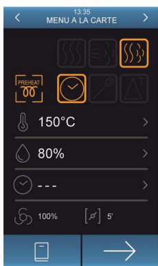
Screen for setting the cooking type/temperature/humidity/ventilation for the entire cycle. Alternatively, the recipe can be retrieved from the recipe book.
